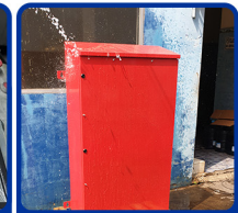
TEST IP PANEL
